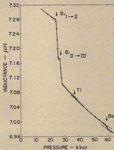
FIG. 11. The inductance of the coil on a compound core of concentric cylinders of bismuth (80%), thallium (10%), and barium (10%).
